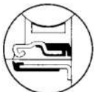
1000GFS With spherical outside diameter and integral set screw lock
