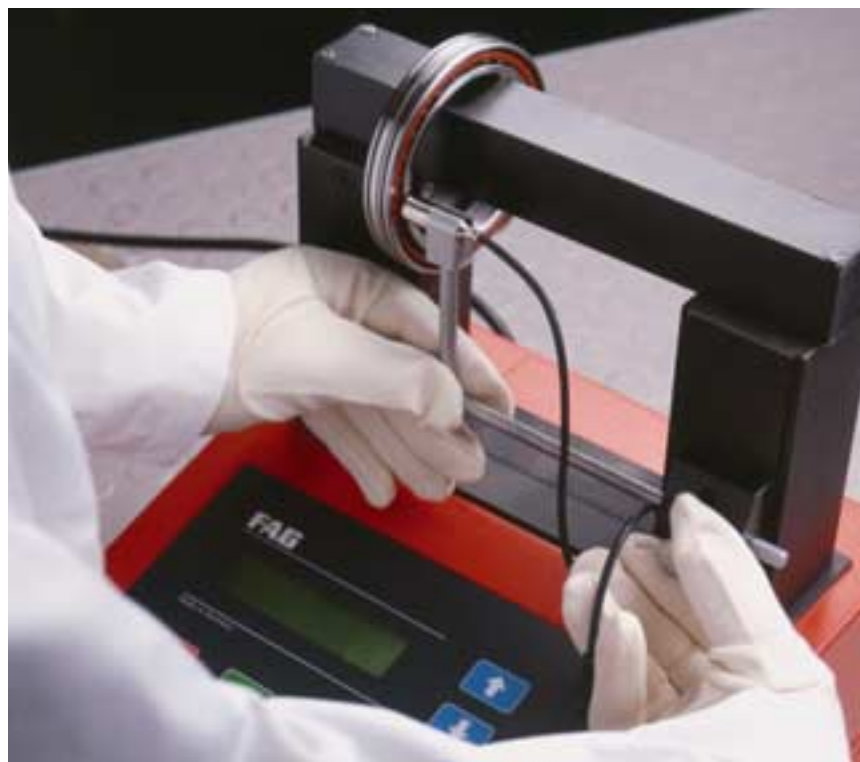
40: Mounting using an induction heating device
